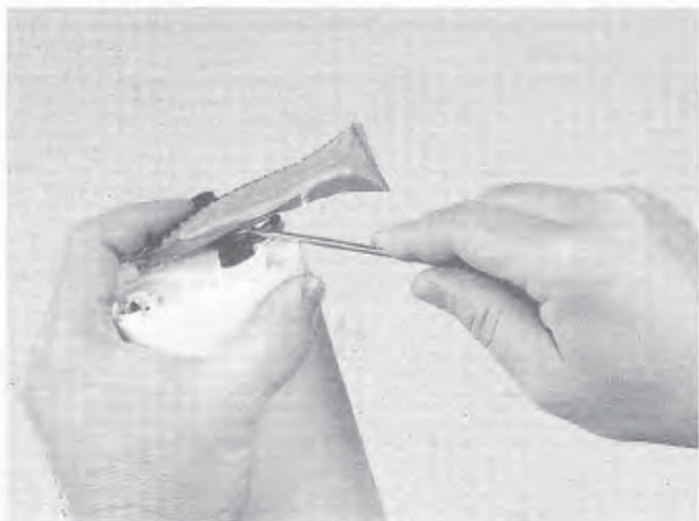
7.6 The strainer and its O-ring can be carefully pulled from the module
