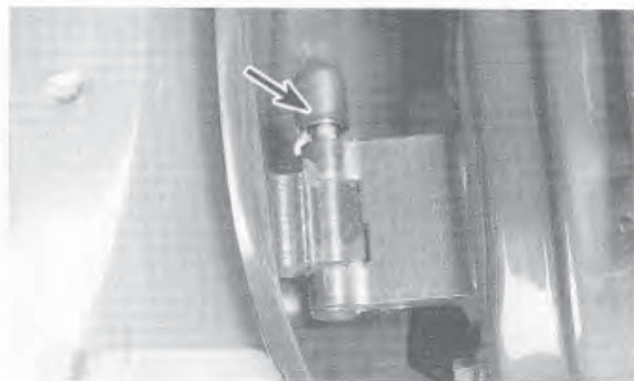
16.4b Remove the upper cover (arrow) and drive the hinge retaining sleeve upward to remove it
