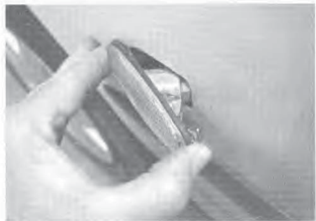
14.1 Prise the rear edge out and rotate the side turn signal housing out of the body
