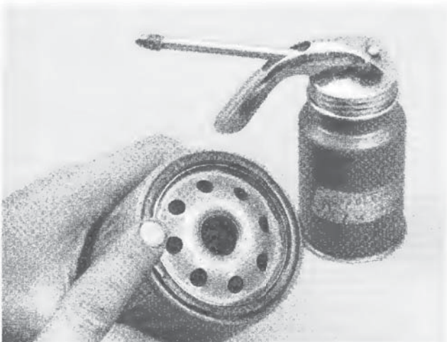
8.12c Lubricate the oil filter gasket with clean engine oil before refitting the filter on the engine
