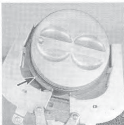
23.12 Refitting the compression rings with a ring expander - the mark (arrow) must face up
