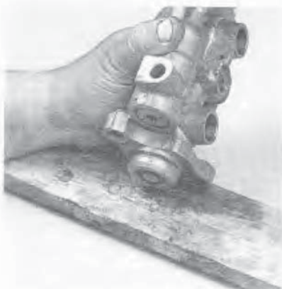
6.8 Use a block of wood to tap out the secondary piston
