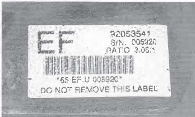
16.7 All rear axle assemblies have an identification label affixed to them
