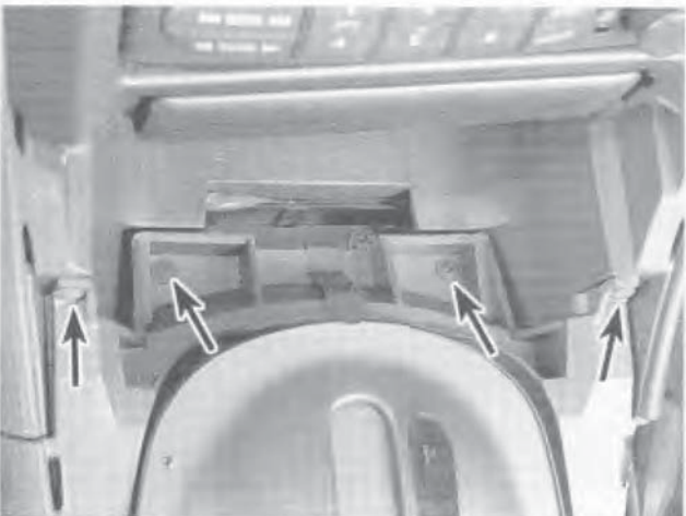
20.4b ... then remove the four screws (arrows) retaining the console to the instrument panel cover
