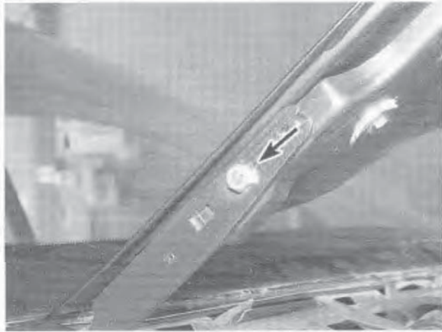
9.4 Remove the bolt (arrow) on each side of the bonnet
