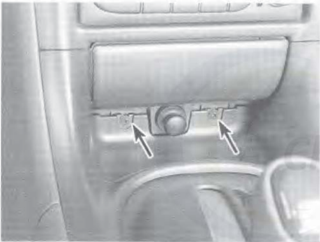
20.4a Remove the screws (arrows) and detach the ashtray cover ...
