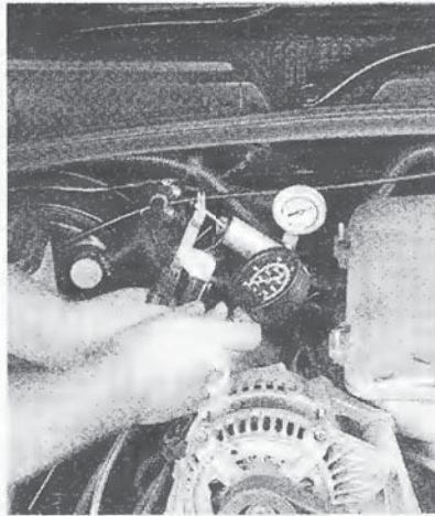
3.18b Next, apply vacuum to the fuel pressure regulator and check the fuel pressure - the fuel pressure should decrease as the vacuum increases
