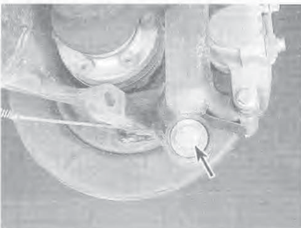
10.3 Remove the lower shock absorber bolt (arrow)
