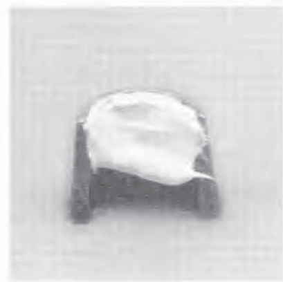
6.16 Apply a small dab of grease to each collet as shown here before refitting - it'll hold them in place on the valve stem as the spring is released
