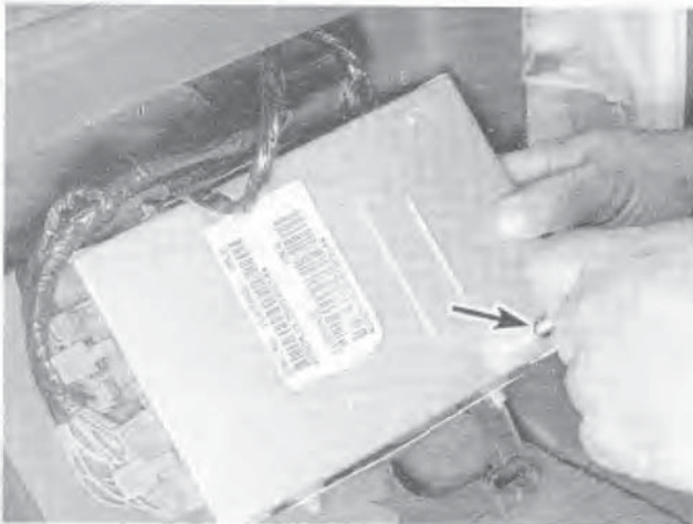
3.9 Remove the two screws and the PROM access cover from the PCM
