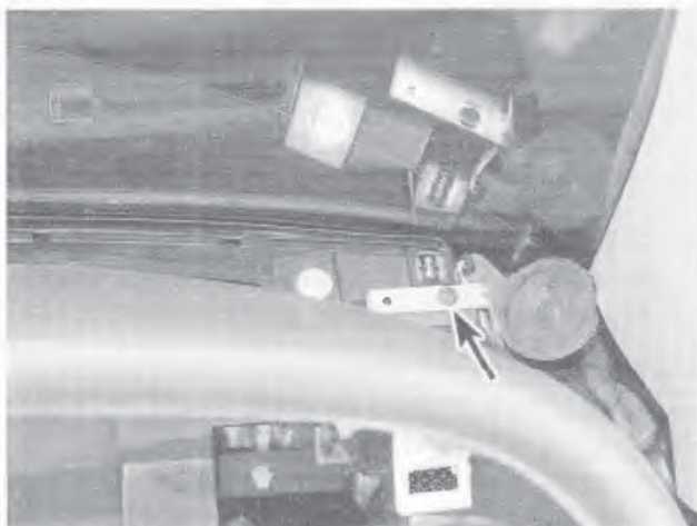
15.6 Remove the instrument panel mounted speaker screw (arrow)
