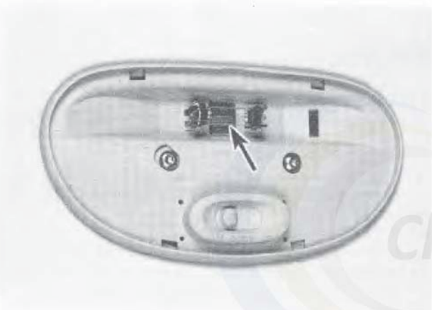
14.23 Pull the bulb (arrow) from the terminals
