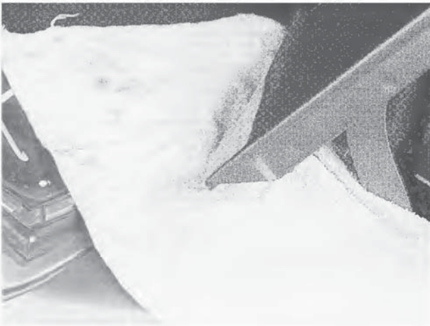
9.1 Pad the back corners of the bonnet with rags so the paint or the windscreen won't be damaged if the bonnet accidentally swings rearward
