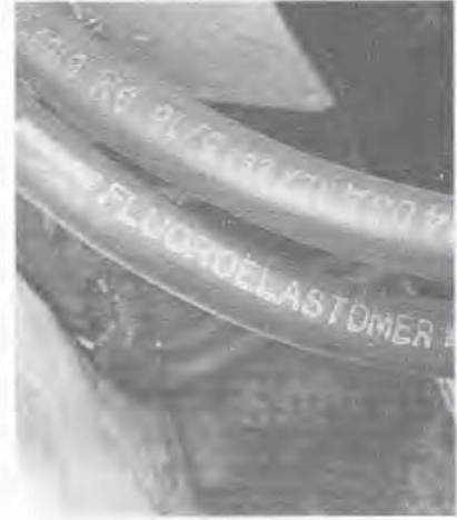
4.8 Correct fuel hose is always clearly marked. Don't use any other type in the fuel system
