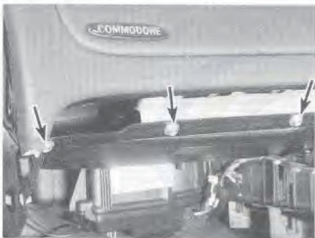
23.4c Remove the insulation panel screws (arrows)
