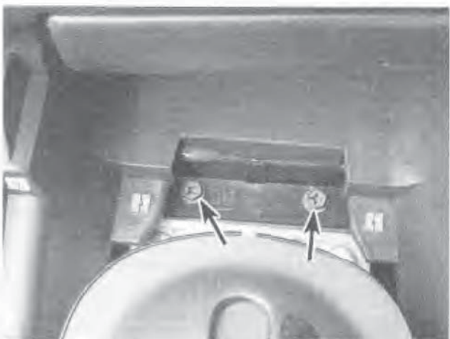
23.9a Remove the screws (arrows) securing the bottom of the centre fascia
