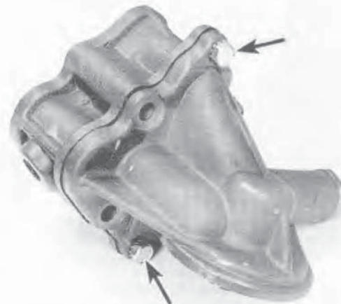
13.5 Remove the remaining two bolts (arrows) which secure the housing of the pump to the pump cover
