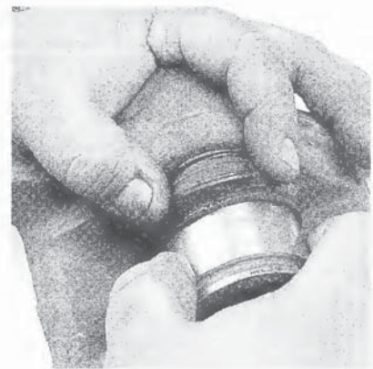
4.12 Slip the boot over the piston and push the piston to the bottom of the bore
