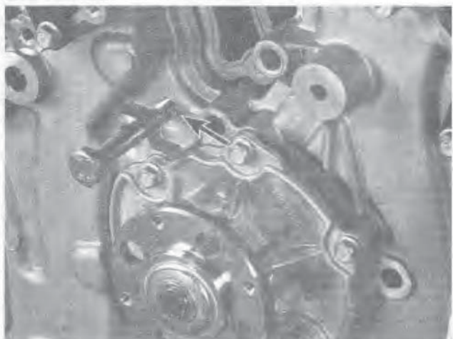
12.9b A 10 x 1.5 mm bolt can be used at the illustrated point, near the water pump to press the centre portion of the cover away from the engine.
