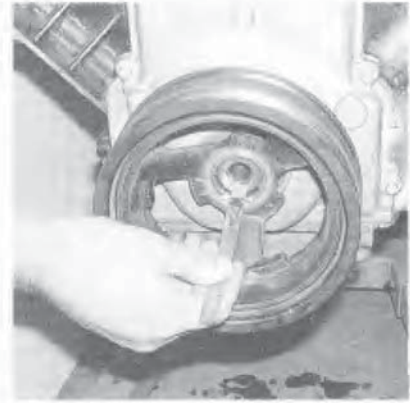
10.9 Before the new crankshaft bolt is fitted and tightened, the balancer must be measured for proper depth - when properly refitted, the balancer hub should extend 2.40 to 4.48 mm past the crankshaft snout
