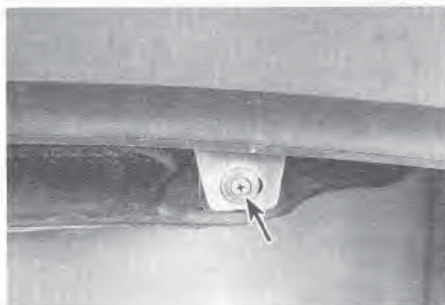
14.8a Remove the two plastic rivets (arrow) on the bottom of the rear bumper
