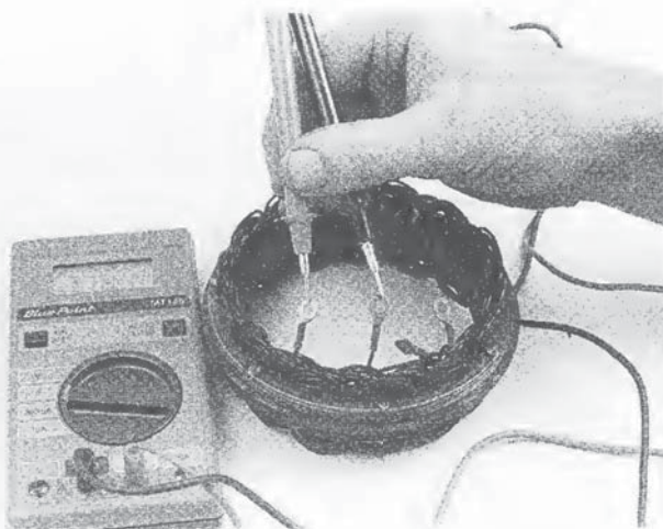
14.16a Check for continuity between each of the stator terminals...
