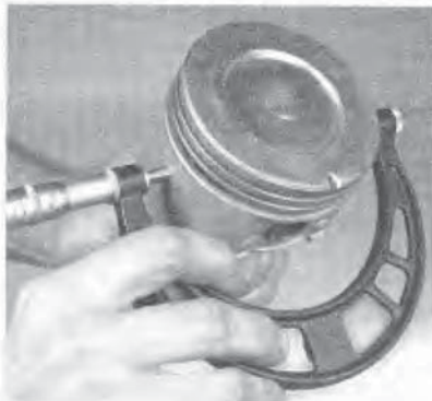
19.11 Measure the piston diameter at a 90-degree angle to the piston pin and in line with it
