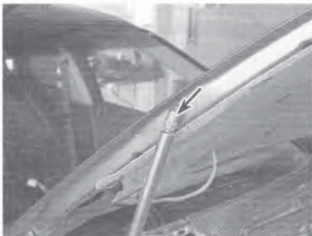
11.2a Use a screwdriver to detach the clip (arrow) at the end of the strut
