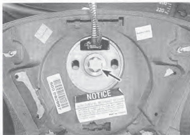
14.5 Remove the steering wheel bolt (arrow), using the special Torx bit
