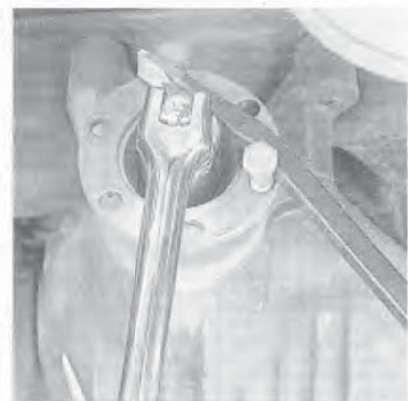
17.5 If you don't have a special holding tool, use a large lever and two bolts to hold the pinion flange from turning while you remove the nut
