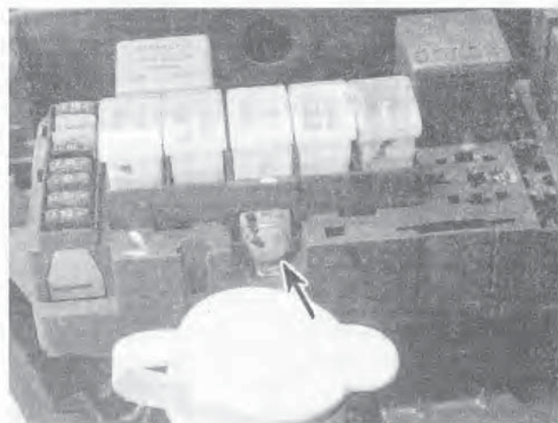
4.1 The fusible links are mounted in the engine compartment adjacent to the fuse block. The main fusible link is retained by a bolt (arrow)
