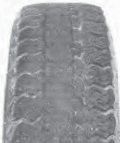
INCORRECT TOE-IN OR EXTREME CAMBER
