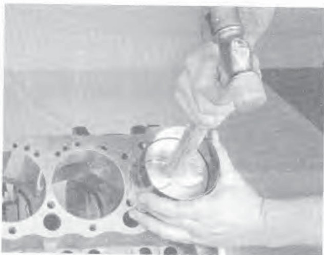
27.11 Drive the piston into the cylinder bore with the end of a wooden or plastic hammer handle
