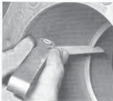
23.4 With the ring square in the cylinder, measure the end gap with a feeler gauge
