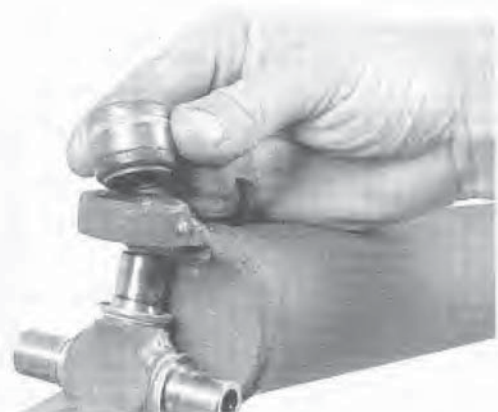
12.4b After it has been pressed out, remove the bearing cup from the yoke ear
