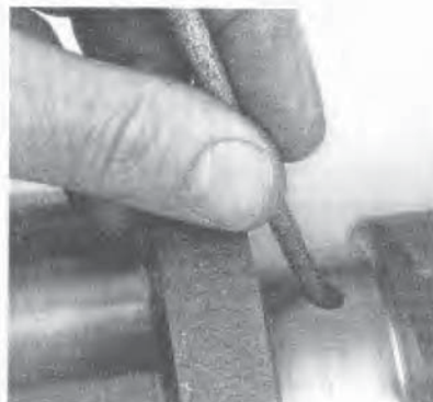
20.1 The oil holes should be chamfered so sharp edges don't gouge or scratch the new bearings
