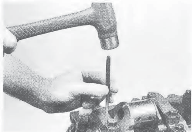
15.4b The arrow on the main bearing cap indicates the front of the engine. Mark the caps to indicate their positions with a centrepunch
