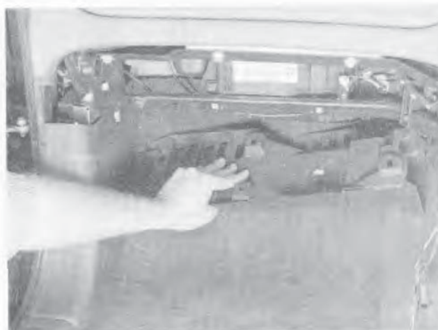
23.14 Detach the upper footwell closing panel by pulling it down and to the left
