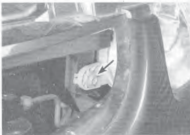
13.4 The headlight housing is held in place by two bolts at the top and one bolt (arrow) at the corner
