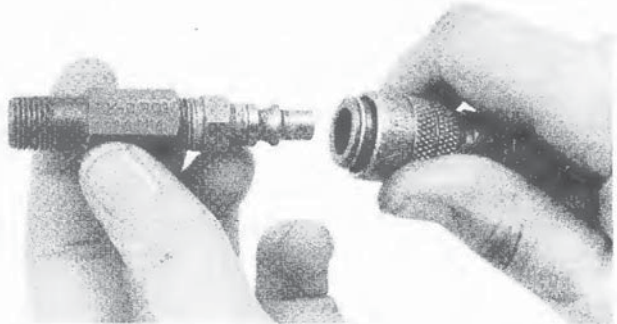
6.4 This is what the air hose adapter that threads into the spark plug hole looks like - they're commonly available from auto parts stores
