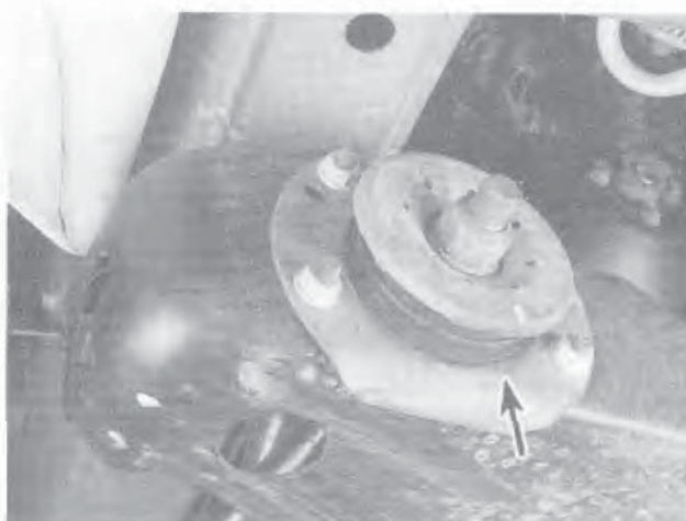
13.6 Inspect the tension rod damper (arrow) for damage and leaking fluid
