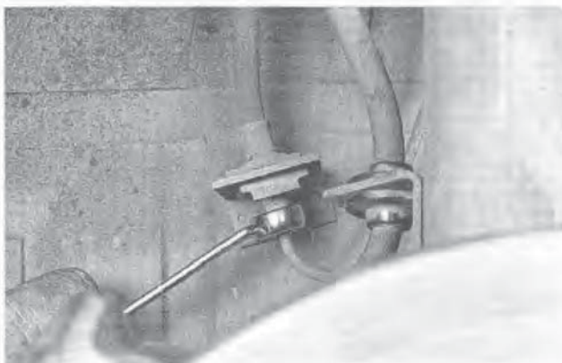
7.2 Using a flare-nut spanner, unscrew the brake line from the hose fitting, being careful not to bend the frame bracket or brake line
