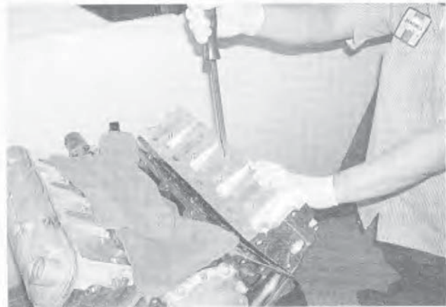
9.8 Using a prisebar inserted into an inlet port to break the head loose - do not use excessive force or damage to the head may result
