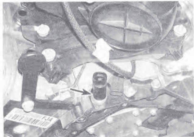
2.4b Oil pressure sending unit location - 5.7 litre Gen III V8 engines
