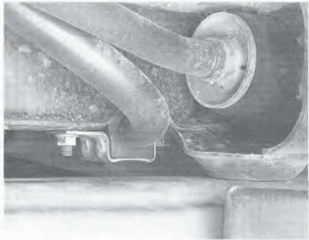
2.3 To detach the stabiliser bar from the frame, remove the bolts and nuts from both bush clamps - make sure the slit in the bush faces forward when you refit the stabiliser bar
