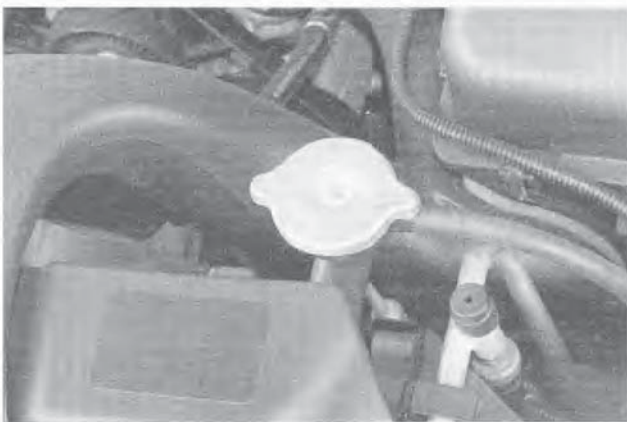
4.9a DO NOT remove the radiator cap unless the engine has thoroughly cooled
