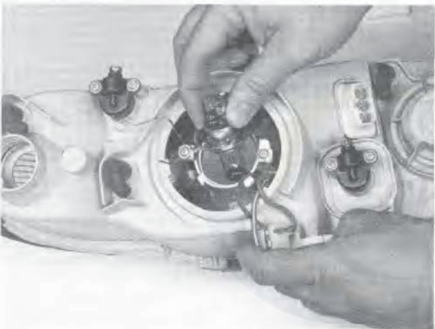
11.4b Withdraw the bulb holder. Don't touch the bulb with your fingers
