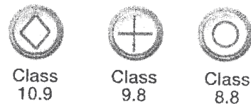
Metric stud strength markings
