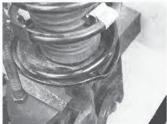
8.16 When refitting the spring, make sure that the end engages in the lower seat like this
