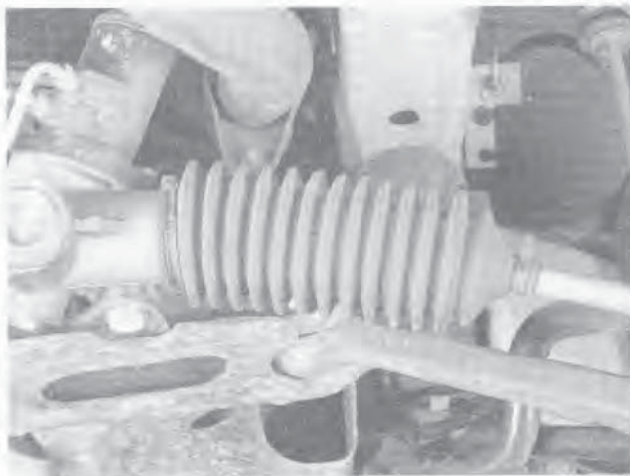
13.4a Inspect the rack-and-pinion steering boots (there's one on each side) for tears or leaking grease
