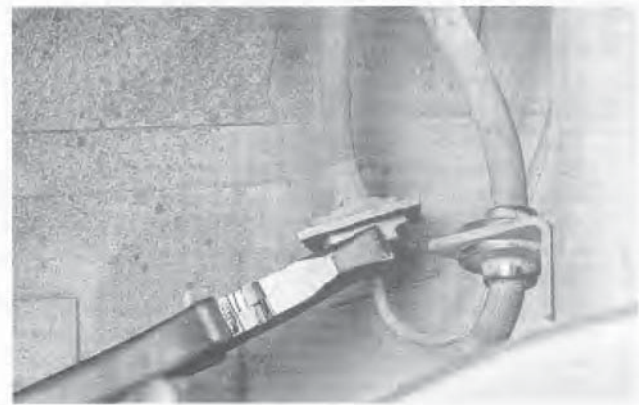
7.3 Use pliers to remove the U-clip from the female fitting at the bracket, then remove the hose from the bracket
