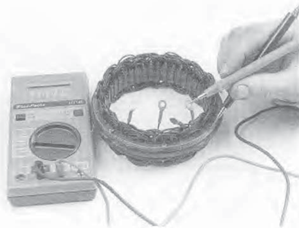
14.16b ... there should be no continuity between the stator terminals and the frame - if there's an open or short in the stator windings, the stator should be renewed
