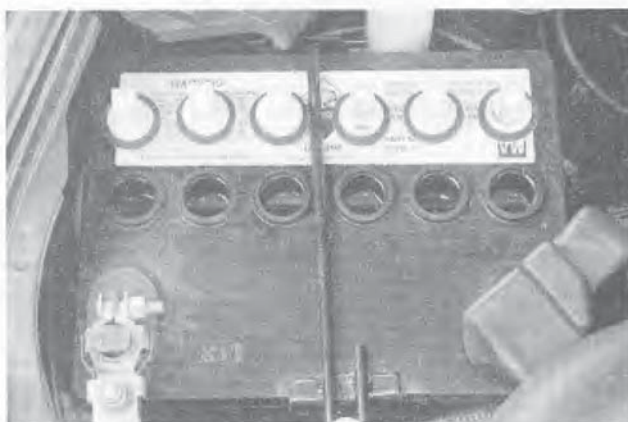
4.16 Remove all six caps and check the level in each one
