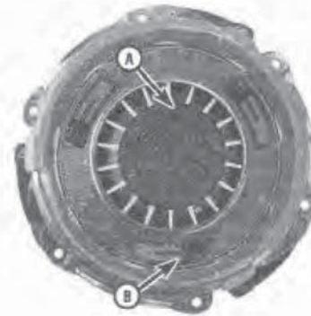
6.17 On 5.7 litre Gen III V8 and 6.0 litre Gen IV V8, press against the pressure plate diaphragm spring illustrated at point A, then slide the stepped adjusting ring fully counter clockwise illustrated at point B
