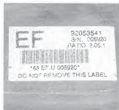
The identification tag and gear ratio tag is found on the left side of the differential housing
