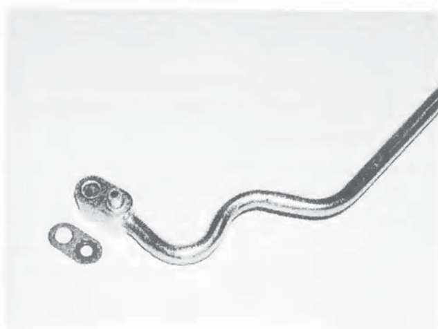
9.18 Be sure to use new gaskets at each cylinder head head-to-vent pipe joint - position the O-ring seal over the vent pipe nipple
