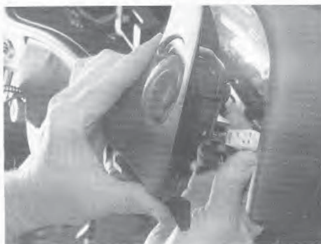
25.4 Grasp the bezel securely and pull out sharply to detach it, then unplug the electrical connectors
