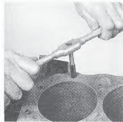
16.8 All bolt holes in the block - particularly the main bearing cap and head bolt holes - should be cleaned and restored with a tap (be sure to remove debris from the holes after this is done)
