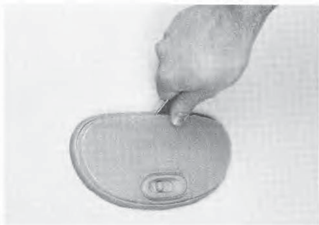
14.22 Use a small screwdriver to detach the interior light lens
