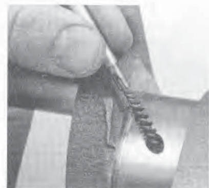
20.2 Use a wire or stiff plastic bristle brush to clean the oil passages in the crankshaft
