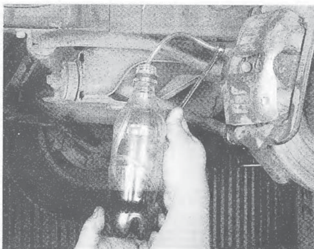
8.6 When bleeding the brakes, a hose is connected to the bleeder screw and then submerged in brake fluid - air will be seen as bubbles in the tube and container (all air must be expelled before moving to the next brake or component)
