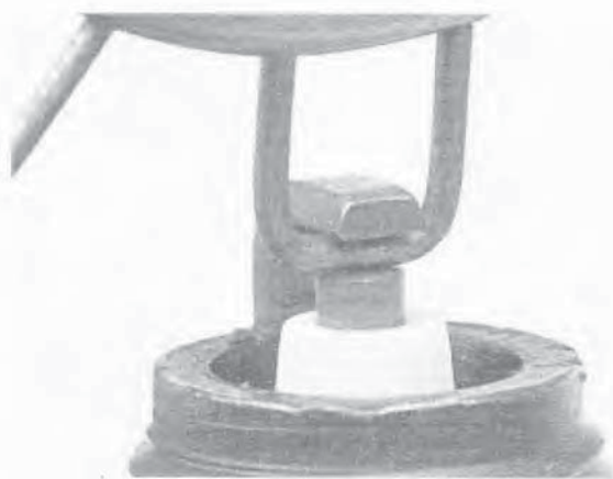
33.5a Spark plug manufacturers recommend using a wire type gauge when checking the gap - if the wire does not slide between the electrodes with a slight drag, adjustment is required
