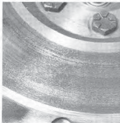
6.8 This flywheel shows signs of wear - it should be resurfaced
