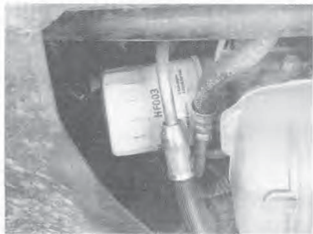
8.12a The oil filter is usually on very tight as well. It will require a special wrench for removal - DO NOT use the wrench to tighten the new filter!
