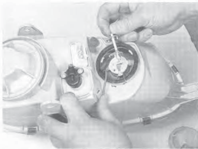
11.8b Pull the bulb straight out of the opening
