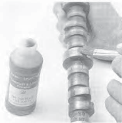
25.1 Be sure to pre-lube the camshaft bearing journals and lobes before refitting
