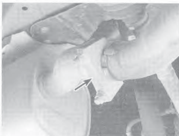
14.2b Inspect the clamps to make sure they are secure
