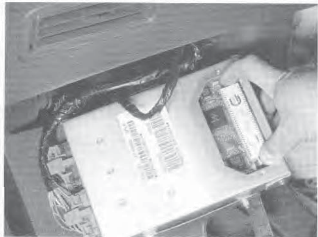
3.10 Using your thumb and finger, press the PROM carrier retainers in and pull the PROM straight up
