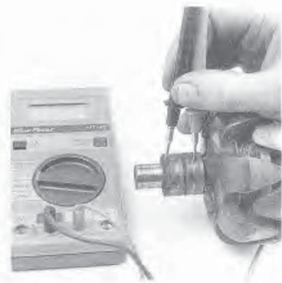
14.14 Check for continuity between slip rings with an ohmmeter. There should be no continuity between either slip ring and the rotor shaft
