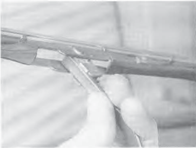
12.5 Depress the release lever, then slide the blade assembly out of the hook in the end of the wiper arm
