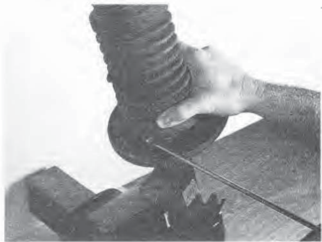
8.14a Loosen the dust boot clamp with a screwdriver ...
