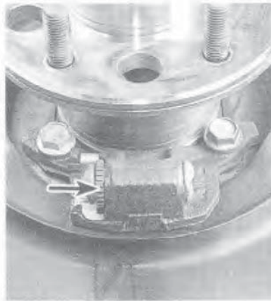
10.4b ... and use a screwdriver to turn the star wheel adjuster and back off the parking brake shoes
