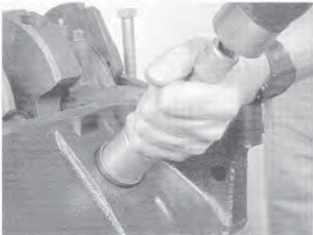
16.10 A large socket on an extension can be used to drive the new core plugs into the bores
