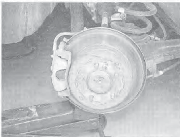
11.5 Put a floor jack under the rear of the control arm before removing the shock absorber
