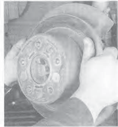
10.4c Remove the rear disc and parking brake drum assembly
