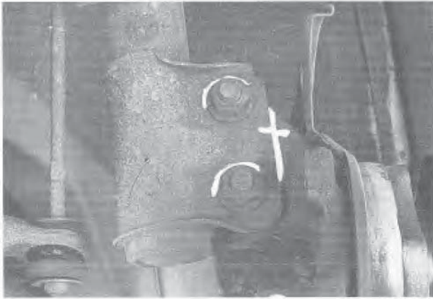
6.6 Mark the strut-to-steering knuckle relationship, then remove the bolts
