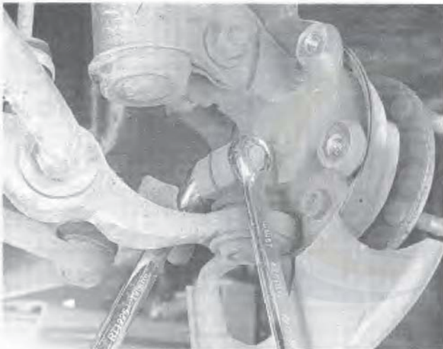
3.3 Use two spanners to remove the balljoint clamp bolt and nut
