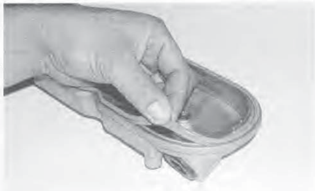
4.12 Position the new gasket in the valve cover lip
