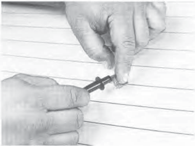
17.4 When measuring voltage at the defogger grid, wrap a piece of tin foil around the negative probe of the voltmeter and press the foil against the wire with your finger
