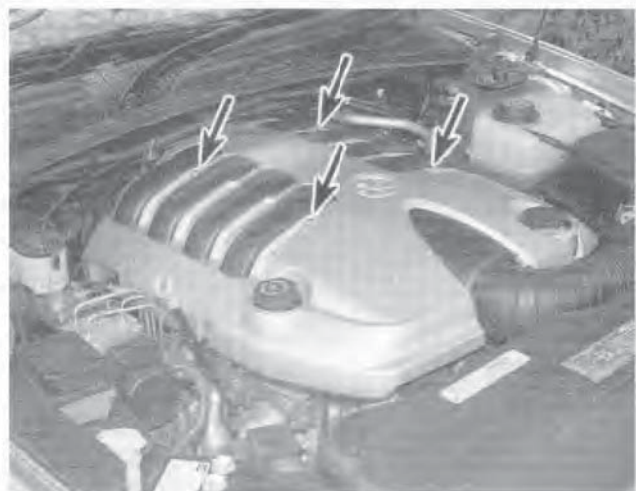
4.2 Remove the engine cover retaining nuts (arrows) and remove the cover
