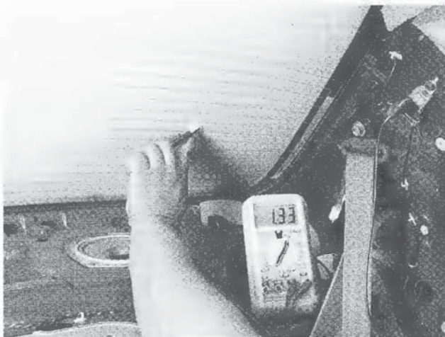
17.7 Slide the probe along the element. It is broken at the point where the voltmeter reading changes sharply
