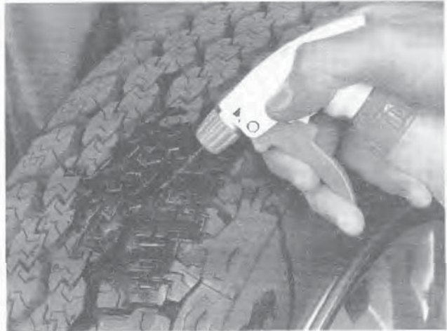
5.4b If the valve core is tight, raise the corner of the vehicle with the low tyre and spray a soapy water solution onto the tread as the tyre is turned slowly - leaks will cause small bubbles to appear
