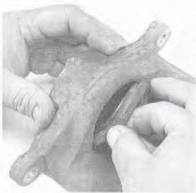
4.6 Remove the dust boot from the caliper
