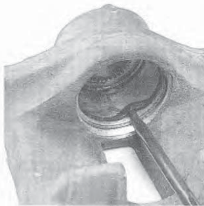
4.7 The piston seal should be removed with a plastic or wooden tool to avoid damage to the bore and the seal groove (a pencil will do the job)
