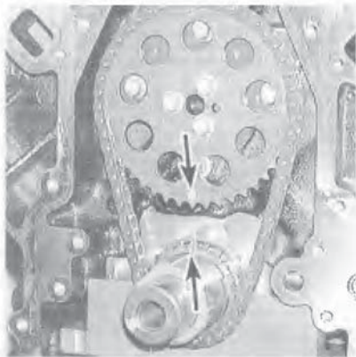
12.9 Timing chain alignment marks (arrows) - when properly aligned, the crankshaft gear should be in the 12 o'clock position, the camshaft gear should be in the 6 o'clock position and the number one piston should be at TDC
