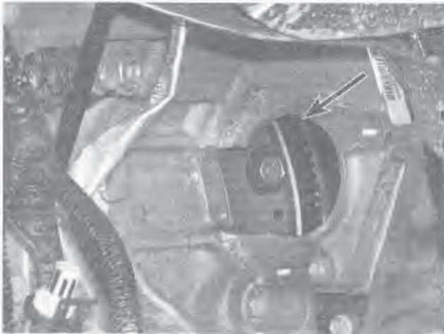
10.4 Place a lever between the ring gear teeth and the cylinder block to hold the crankshaft while removing the centre bolt
