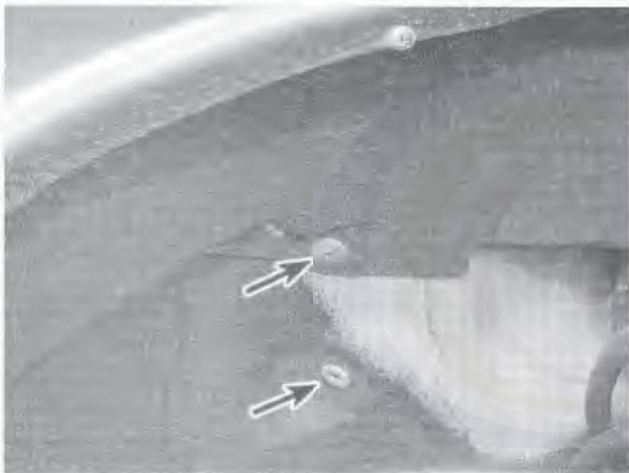
13.2 Remove the plastic screw fasteners (arrows) and detach the fender liner
