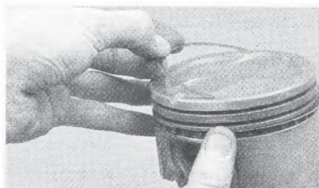
23.9b DO NOT use a piston ring refitting tool when refitting the oil ring side rails
