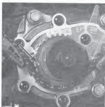
12.10 Crankshaft sprocket in correct position
