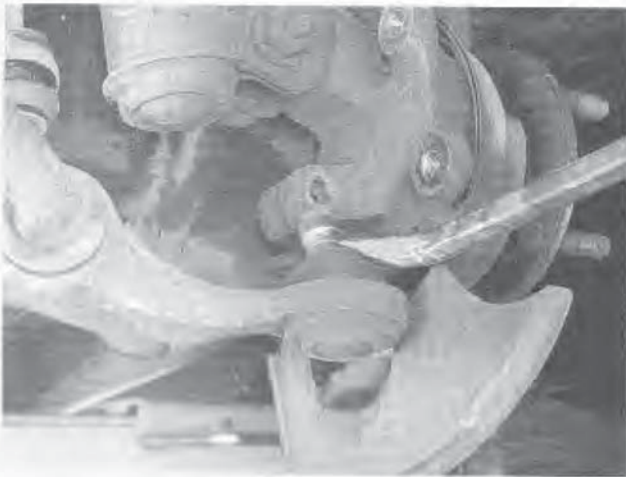
3.6 To separate the lower control arm from the steering knuckle, insert a lever between the control arm and the knuckle as shown
