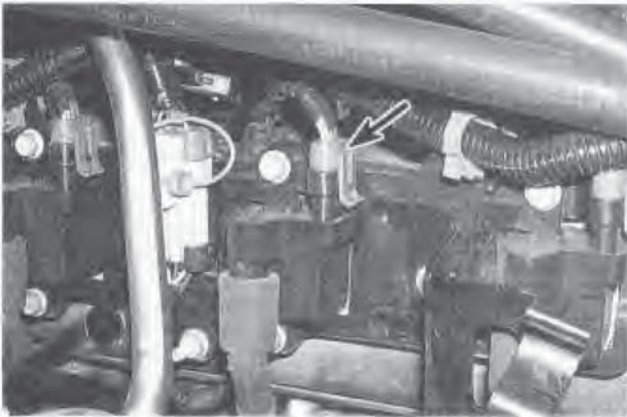
7.4 Disconnect an ignition coil electrical connector (arrow) and check for battery power at the pink wire terminal of the connector
