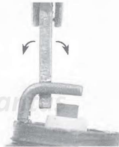
33.5b To change the gap, bend the side electrode only, as indicated by the arrows, and be very careful not to crack or chip the porcelain insulator surrounding the centre electrode
