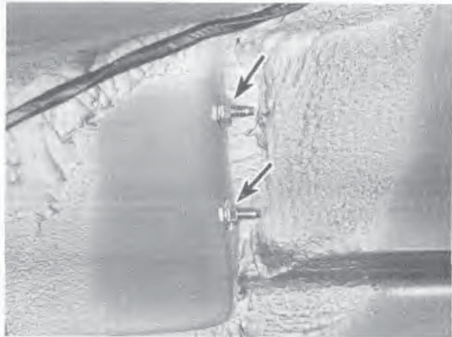
14.10 Open the luggage compartment for access to the four rear bumper nuts (arrows, two shown)
