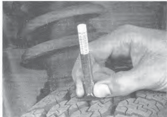
5.2 Use a tyre tread depth gauge to monitor tyre wear - they are available at auto parts stores and service stations and cost very little
