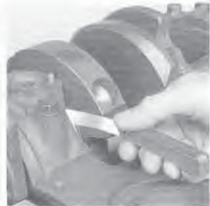
15.3 Checking crankshaft endplay with a feeler gauge
