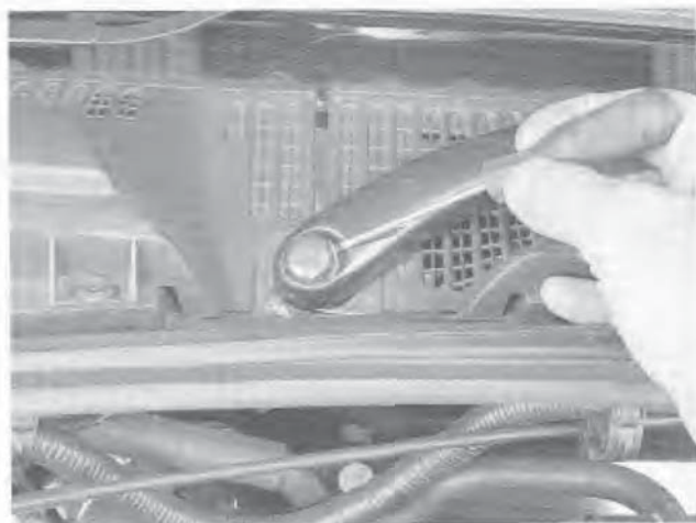
26.1 Prise out the cap with a small screwdriver and remove the nut, then detach the wiper arm
