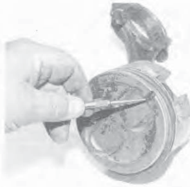
27.9a The notch or arrow on each piston must face the front end of the engine as the pistons are refitted
