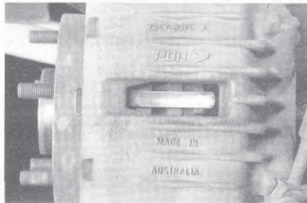
20.5 Look through the opening in the caliper to check the brake pads - the pad lining, which rubs against the disc, can also be inspected by looking through each end of the caliper
