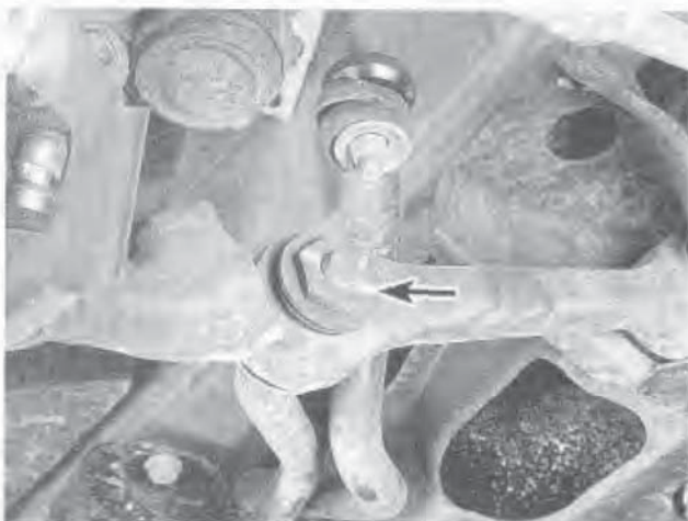
4.3 Remove the tension rod nut and washer (arrow) from the lower control arm
