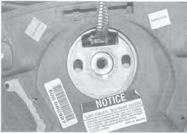
14.6 After removing the steering wheel bolt, use a marking pen to mark the relationship of the steering wheel to the steering shaft
