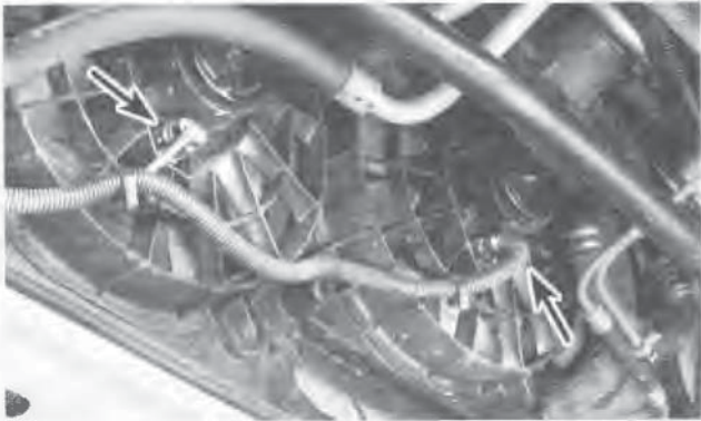
4.1a Locations of the fan connectors (arrows) on twin cooling fan applications
