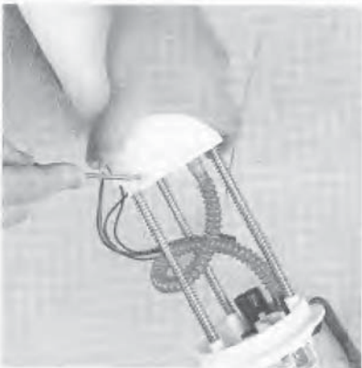
7.8a Use a small screwdriver to push in on the two tangs to release the outer reservoir
