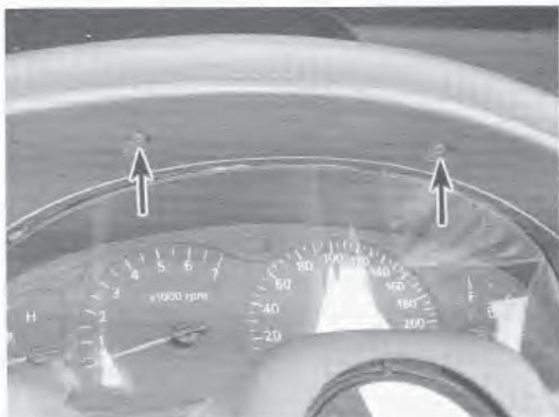
25.3 Remove the two bezel screws (arrows) at the top and five screws along the lower edge of the bezel
