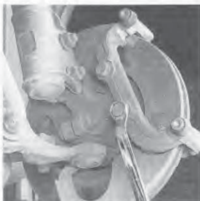
3.4i If the disc is to be removed, remove the bolts and detach the caliper mounting bracket
