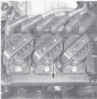
8.10 Pop the wiring retainer (arrow) from the V6 coil pack
