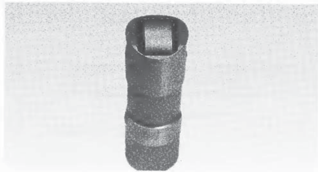
12.20 The roller must turn freely - check for wear and excessive play as well
