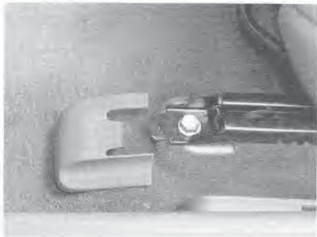
28.2 The front bolts for the front seats can be removed with the seat moved rearward
