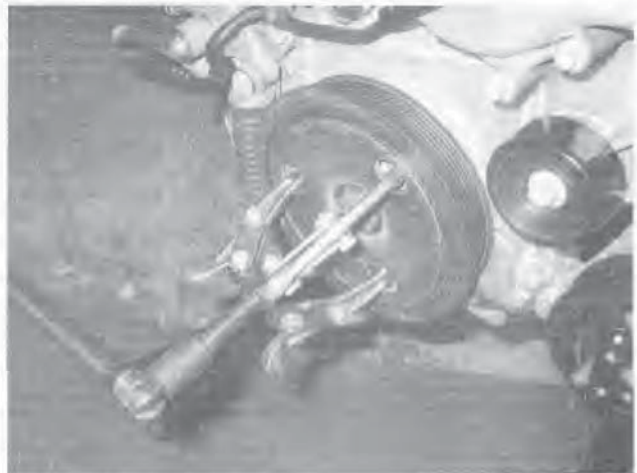
10.5 The use of a three jaw puller will be necessary to remove the crankshaft balancer - always place the puller jaws around the hub, not the outer ring
