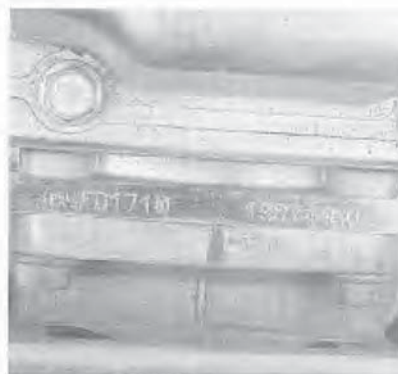
The automatic transmission serial number is visible from below the vehicle
