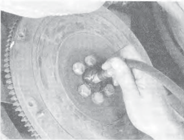
8.8 Fill the cavity behind the bush with grease ...
