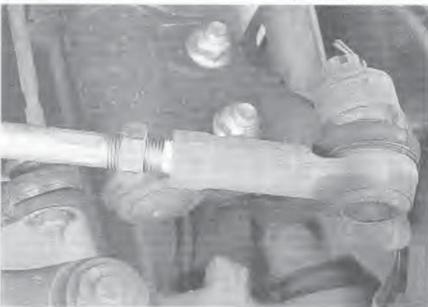
15.2b ... then mark the position of the tie-rod in relation to the threads
