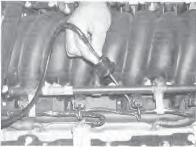
12.8 Use a stethoscope or screwdriver to determine if the injectors are working properly - they should make a steady clicking sound that rises and falls with engine speed changes
