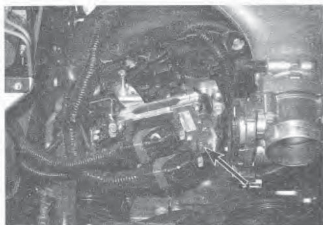
4.7 Slide the grey levers across to disconnect the ECM connectors from the ECM
