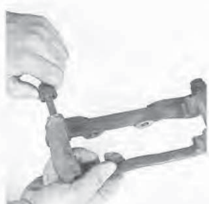
3.4j Pull the caliper guide pins out of their sleeves, clean and inspect them for wear. Lubricate with high temperature grease and refit them in the mounting bracket
