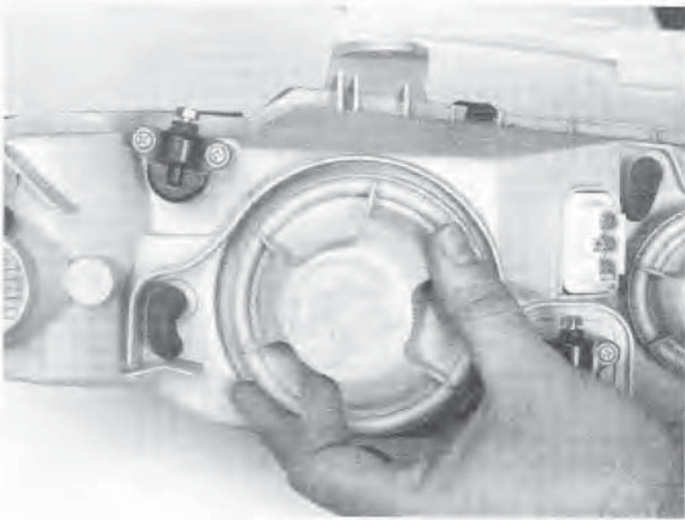
11.2 Remove the headlight bulb cover by rotating it anti-clockwise
