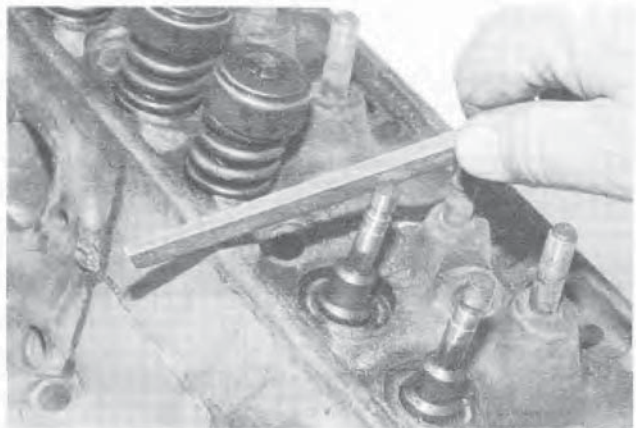
9.4 If the valve won't pull through the guide, deburr the edge of the stem end and the area around the top of the keeper groove with a file or whetstone
