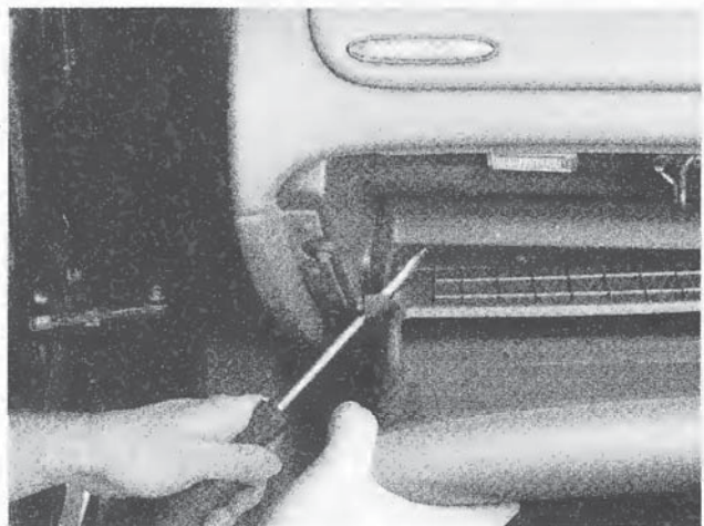
23.4b Using a flat-bladed screwdriver, prise the left side of the glove box out of the dash
