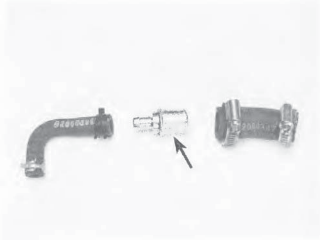
31.7b PCV valve (arrow) and hose component layout (5.0 litre V8 models)
