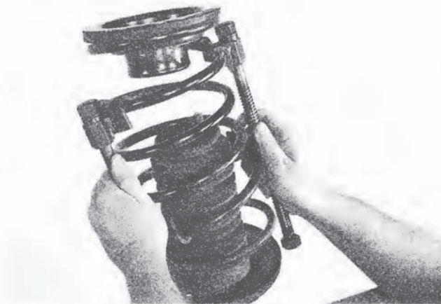
8.9 The spring and compressors can be lifted off the assembly
