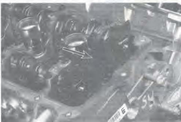
12.23a LH cylinder head with camshaft locking tool fitted
