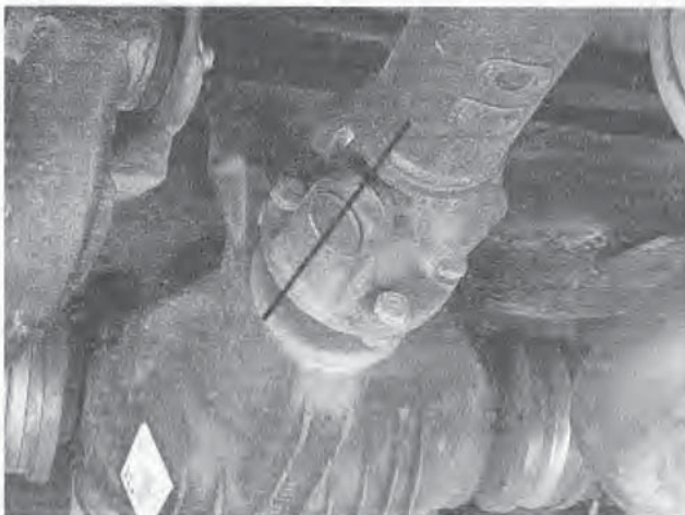
11.3 Scribe a line across the pinion flange, the U-joint and driveshaft so you can later assemble them in the same positions. Use a large screwdriver to hold the shaft from turning while loosening the bolts
