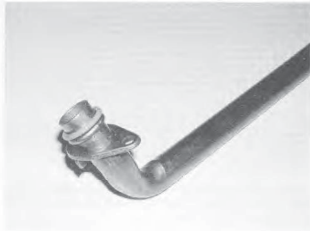
15.8 Always fit a new O-ring on the oil pump pick up tube
