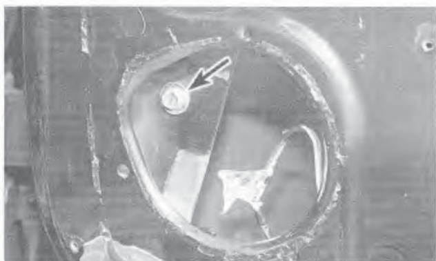
18.2 Remove the bolts retaining the front window guide channel and remove the channel (lower bolt shown)
