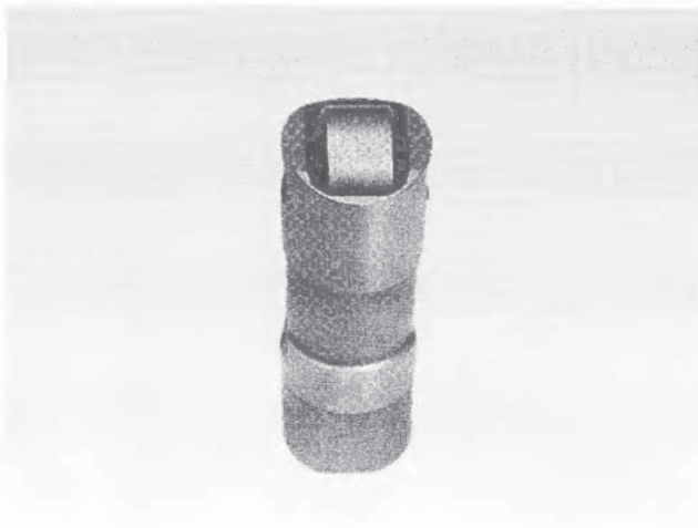
12.23 The roller must turn freely - check for wear and excessive play as well
