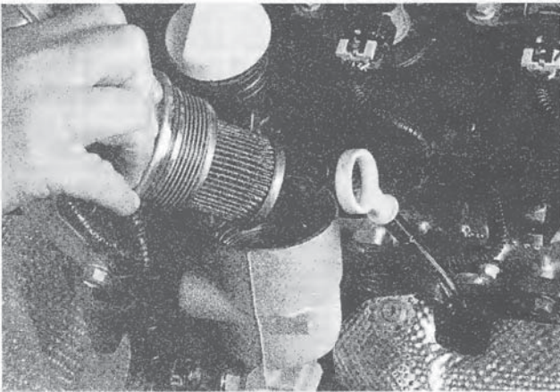
8.13b Removing the cap and oil filter cartridge
