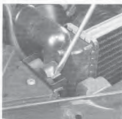
5.9b This view shows the radiator retaining clip disengaged
