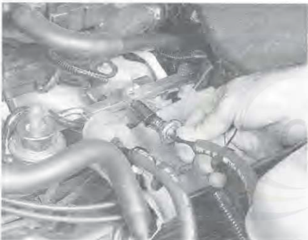
4.13c Insert the fuel line disconnect tool into the line and release the line - 5.7 litre Generation III V8 engine shown
