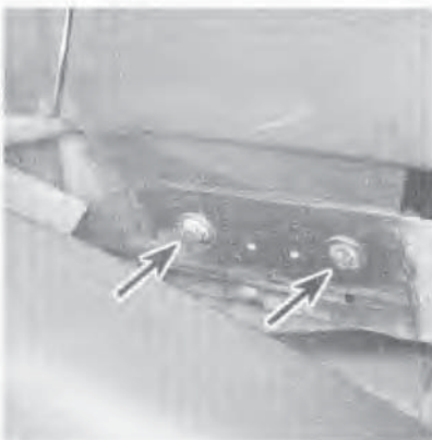
13.3a After detaching the cover, remove the two bolts at the rear lower edge of the fender (arrows), then ...
