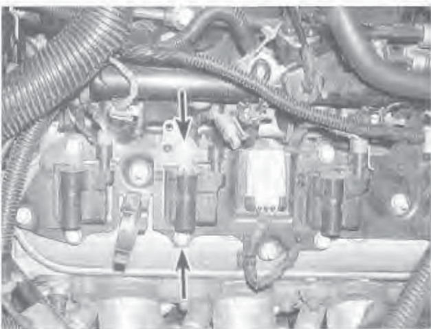
7.23 Remove the ignition coil mounting screws (arrows)
