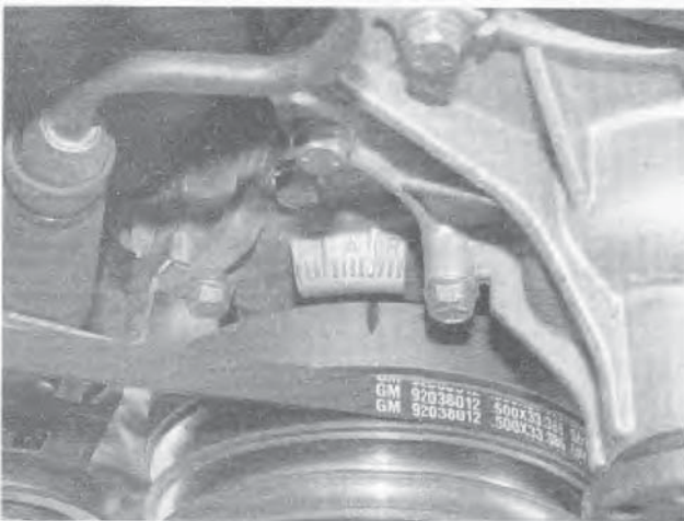
3.6 When the engine is at top dead centre, the mark on the crankshaft balancer will line up with the zero mark (the long line between A and R) mark on the timing indicator
