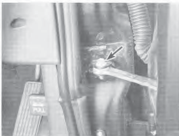
16.3 The door stop assembly can be disconnected by removing the pin or bolt (arrow)
