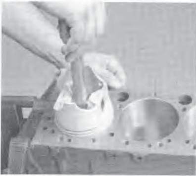
23.3 When checking piston ring end gap, the ring must be square in the cylinder bore (this is done by pushing the ring down with the top of a piston as shown)
