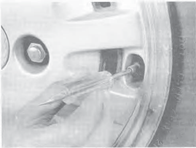
5.4a If a tyre loses air on a steady basis, check the valve core first to make sure it's snug (special inexpensive tools are commonly available at auto parts stores)
