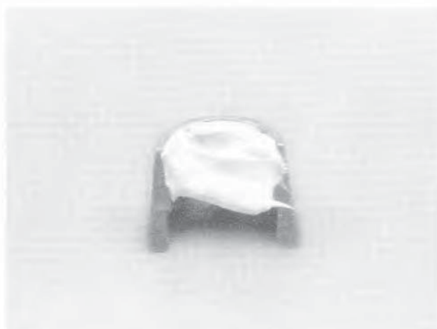
6.16 Apply a small dab of grease to each collet as shown here before refitting - it'll hold them in place on the valve stem as the spring is released
