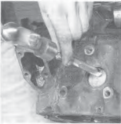
16.4a A hammer and large punch can be used to knock the core plugs sideways in their bores
