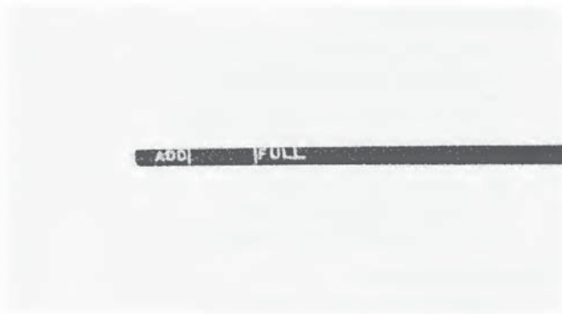
4.4 The oil level should be at or near the upper mark on the dipstick - if it's below the ADD line, add enough oil to bring the level into the upper mark
